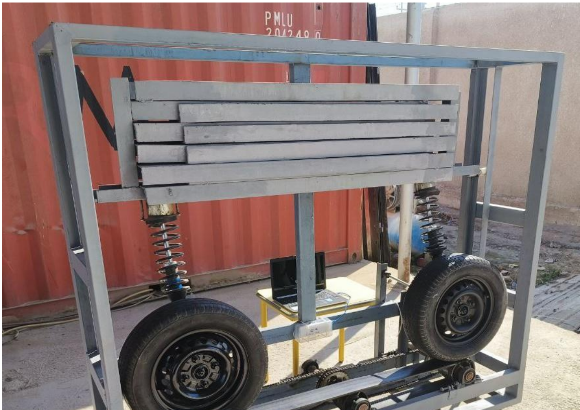
Figure (5-1): A half-automobile model test rig with a single displacement measuring device.
