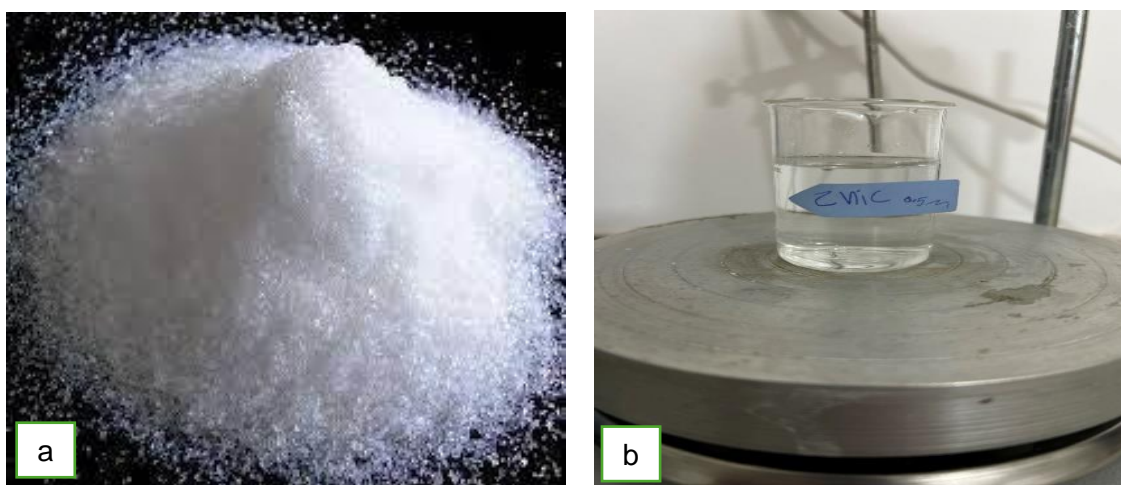
Figure (2.3): Images for Zinc Acetate prepare (a) and the Zinc Acetate solution (b).
