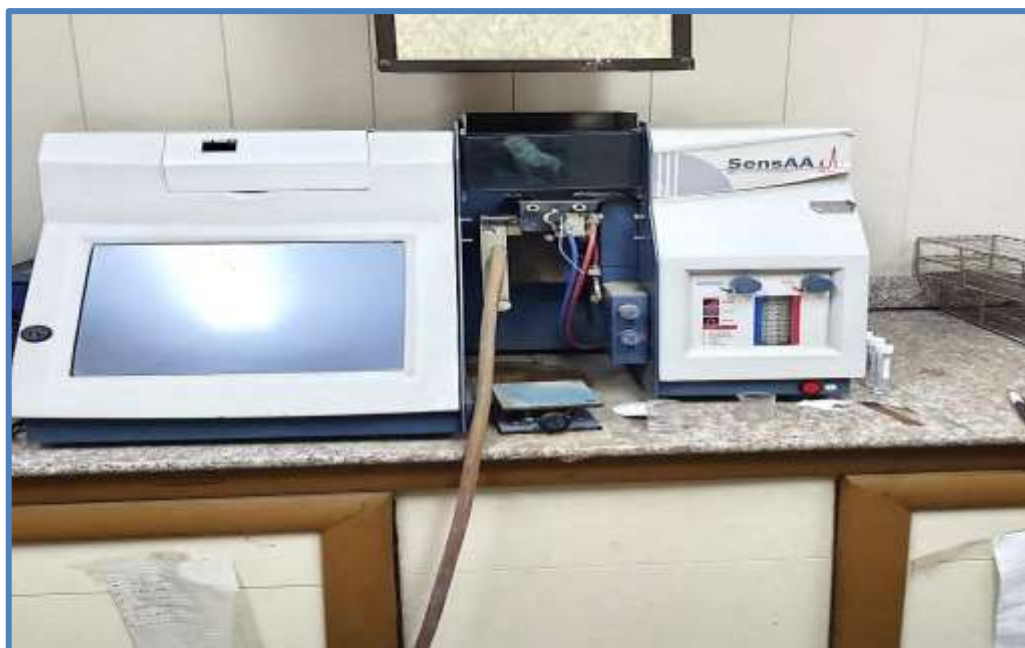
Figure 2-6: Atomic absorption spectroscopy instrument used in this study
