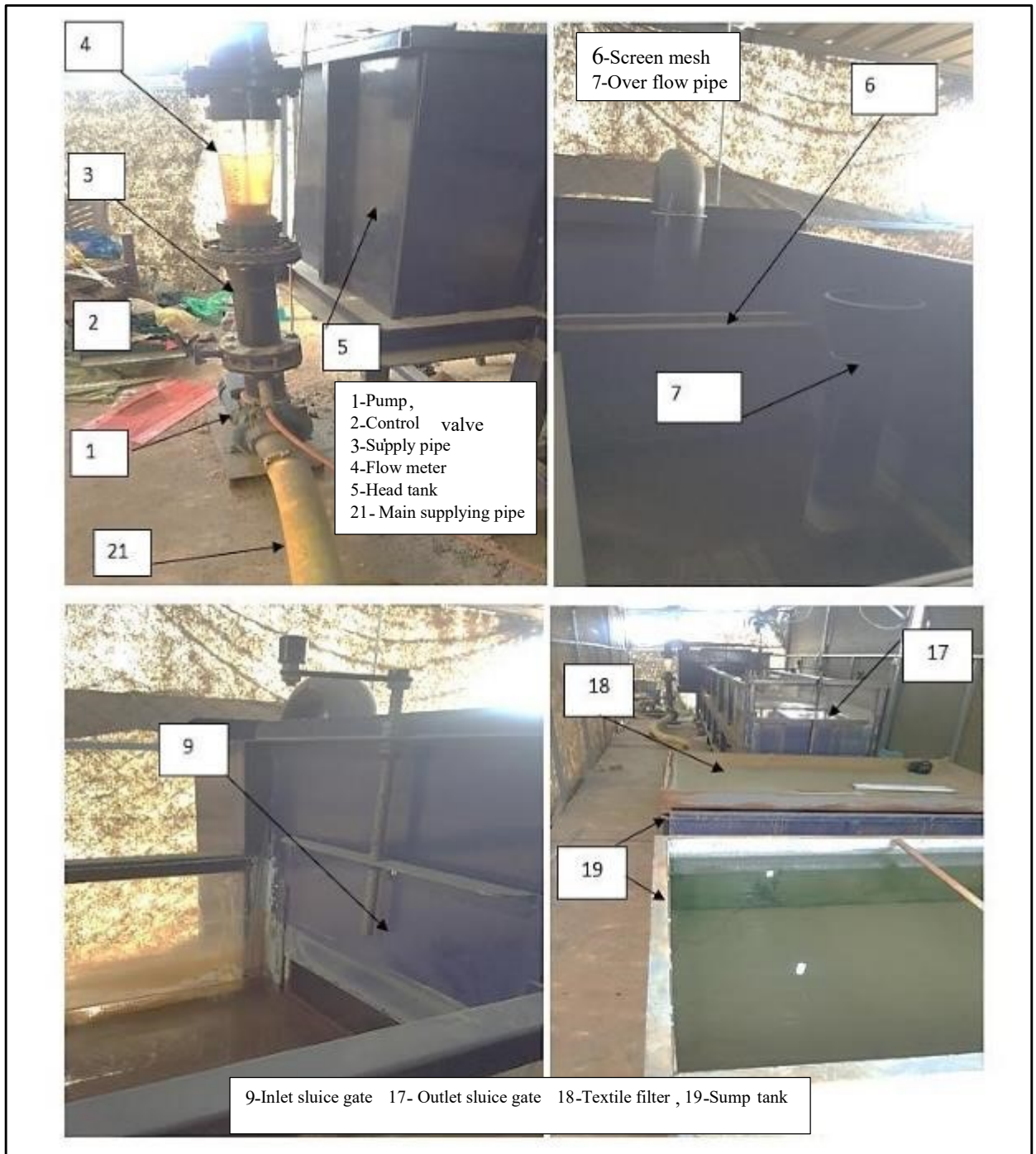
Figure 3-3: Details of the laboratory flume.
