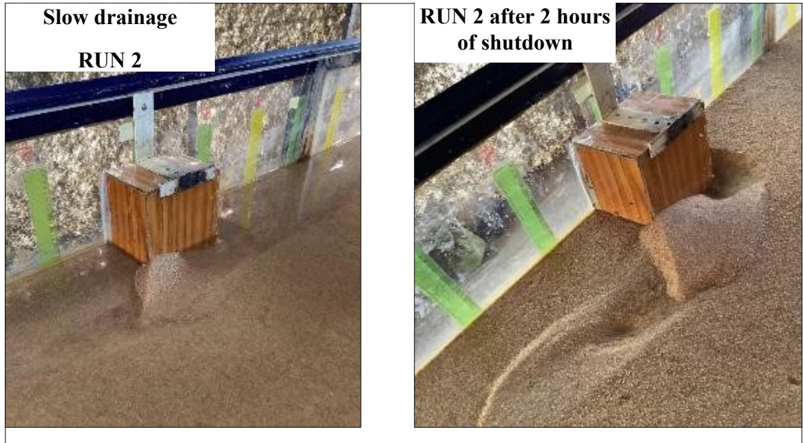
Figure B-4: RUN 2 of Reference tests of the Abutment-A.
