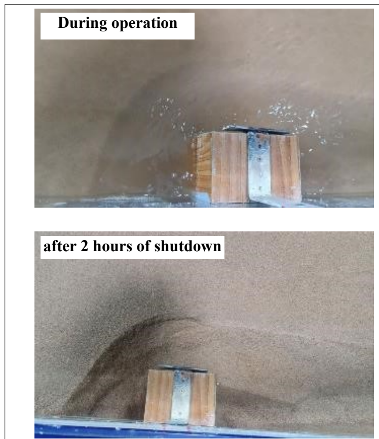
Figure B-5: RUN 4 of Reference tests of the Abutment-A.
