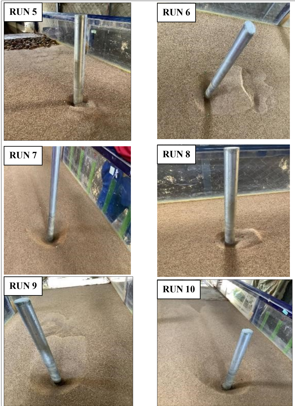
Figure B-2: Reference tests of the pier RUNS( 5-10).
