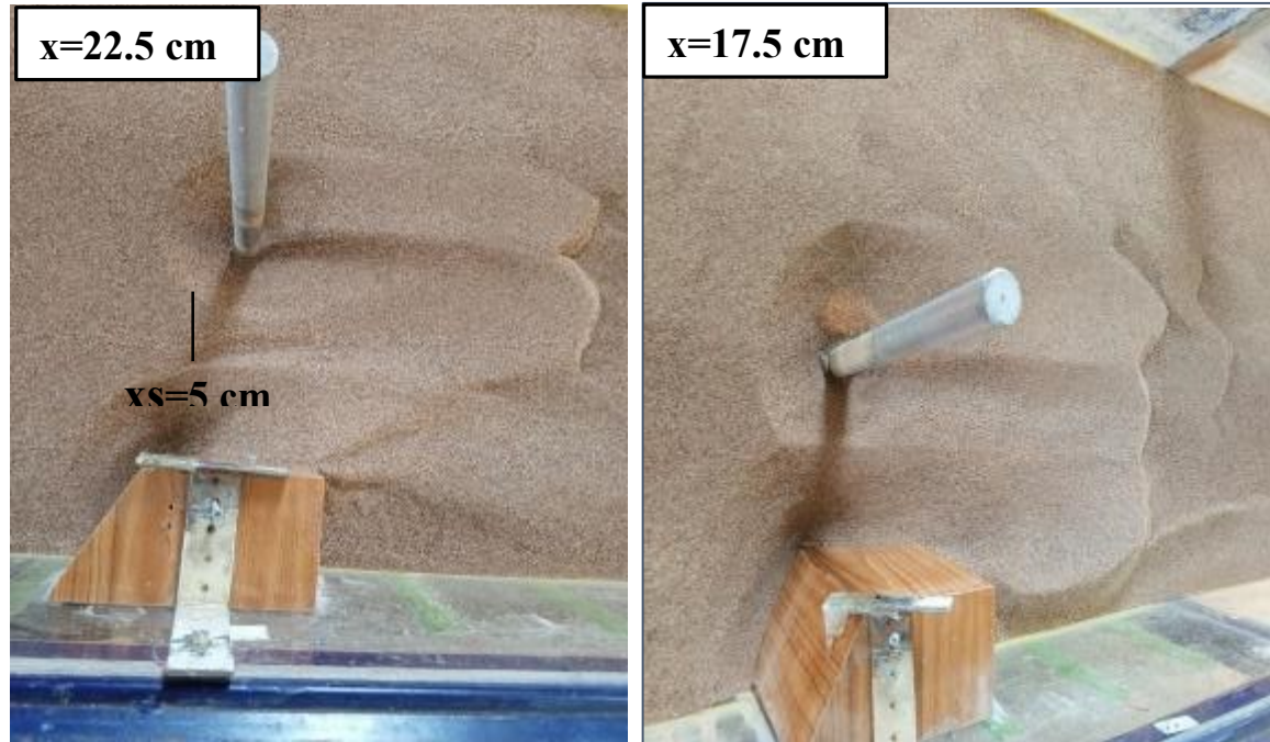
Figure 4-23: The influence of reducing the distance between pier and abutment using the trapezoidal abutment at v/v_c=0.7 .
