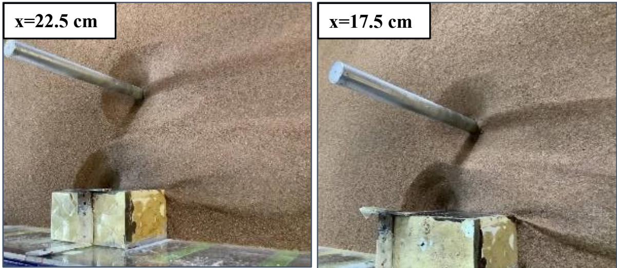
Figure 4-21: The influence of reducing the distance between the pier and abutment using the V3 abutment at v/v_c=0.63 .
