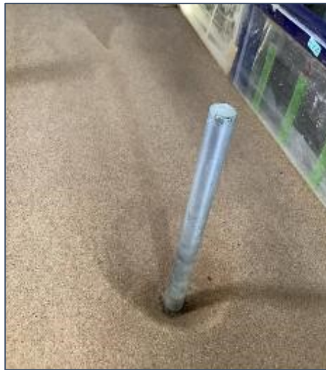
Figure 4-1: Scour hole at v/v_c=0.91 of isolated pier.
