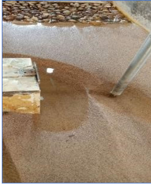
Figure 3-9: Slow drainage of scour holes.
