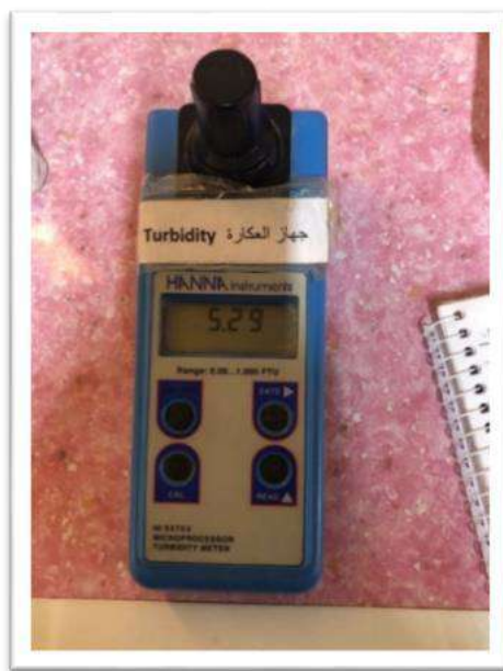
Figure (3-11): Turbidity meter.
