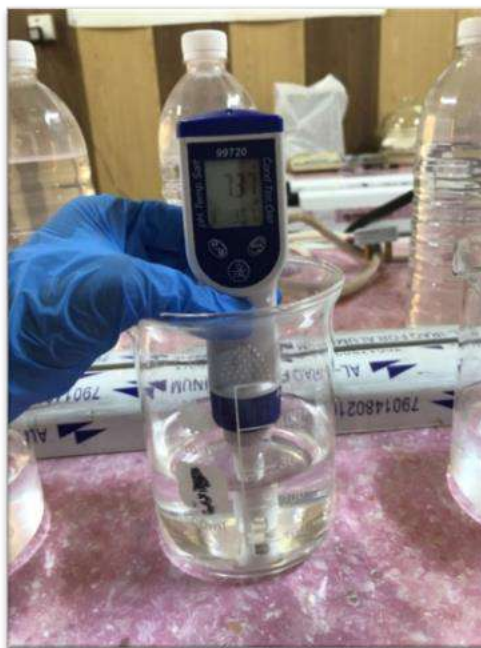
Figure (3-9): PH test.
