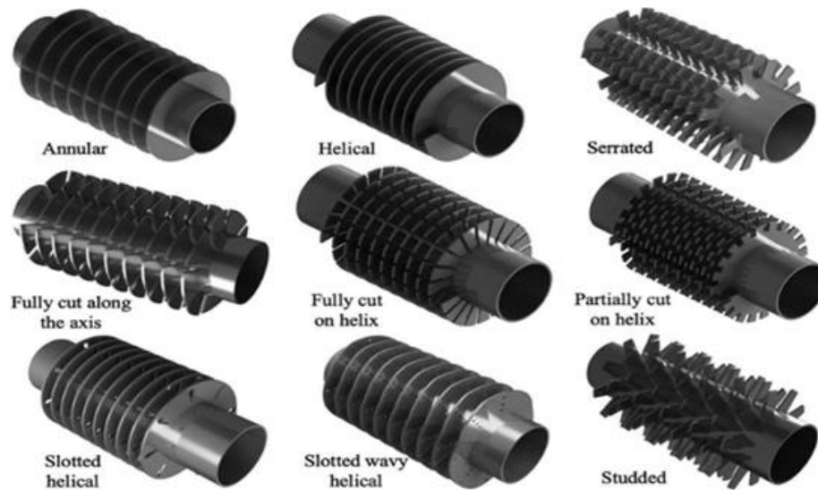
Figure 2.1: Heat Pipes with External Fins Different Shapes [23]
