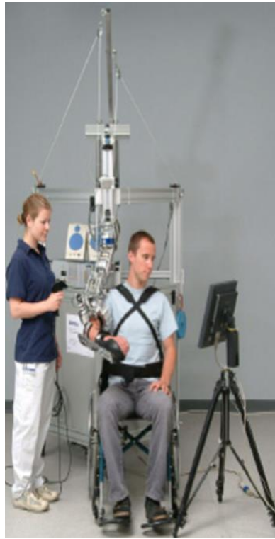
Figure (1.3): Exoskeleton actuated by hydraulic power [2]
